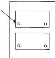
4. Hold the black acrylic sign panel at the desired location on the door or wall and make sure it's level. Pencil in the hole locations onto the wall. Drill 1/8" pilot holes in the center of each hole for the screws and if your wall is hollow insert the wall anchors.
